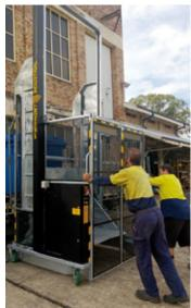
DO **NOT** PUSH ON DOOR - USE SIDE HANDLES WHEN MOVING THE MACHINE.
