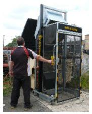
Fill cradle with contents of a wheelbarrow or unruly or loose waste, including bin liner bags containing waste.
