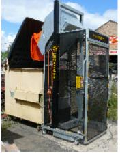
Independently Certified wrightway2MT Bin Tipper. Standard tippers lift up to 240kgs to 1800, 1500 or 1200mm. Custom lift height and weights available to suit specific requirements.
